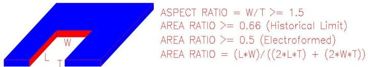
To successfully print small components without reducing the stencil foil thickness, the stencil must be capable of producing acceptable solder paste release at as low a surface area ratio as possible. The historical limit of chemically etched and traditional laser-cut stencils has been a
