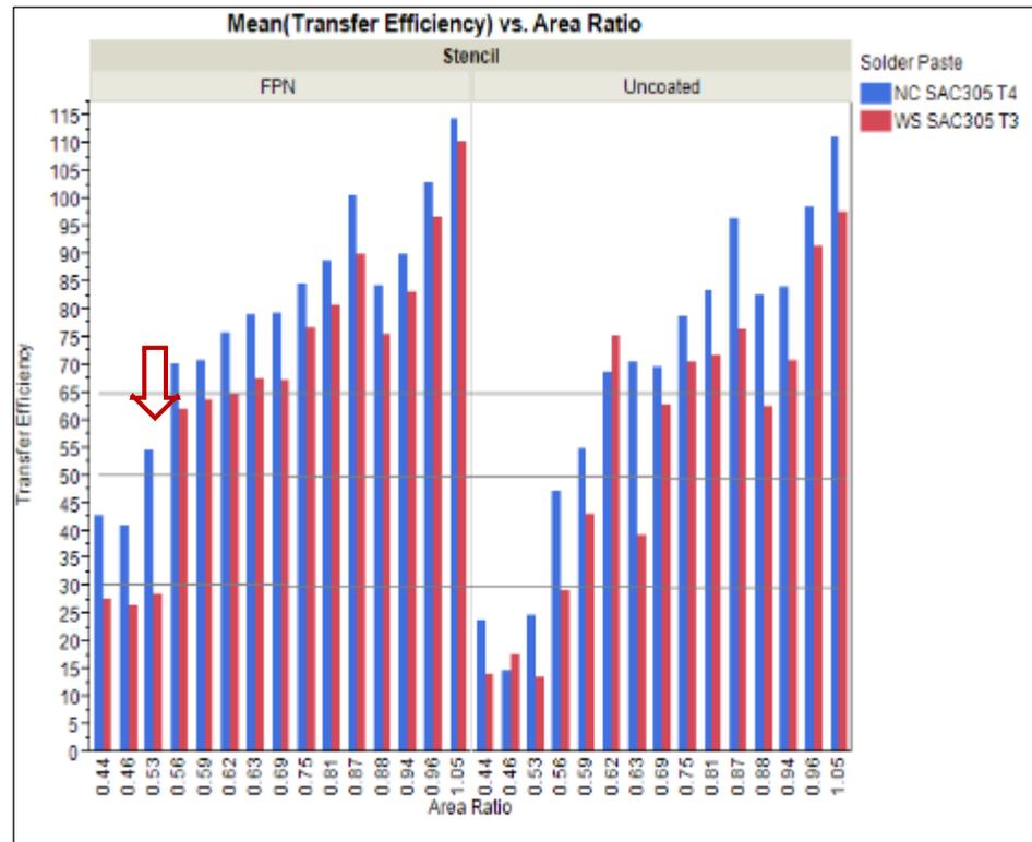
Another indicator of transfer efficiency is solder paste:
