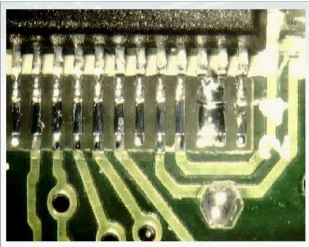
When the PWB land pad is designed for a specific component and the component is replaced by a different component with a shorter foot, bridging at reflow can occur.
