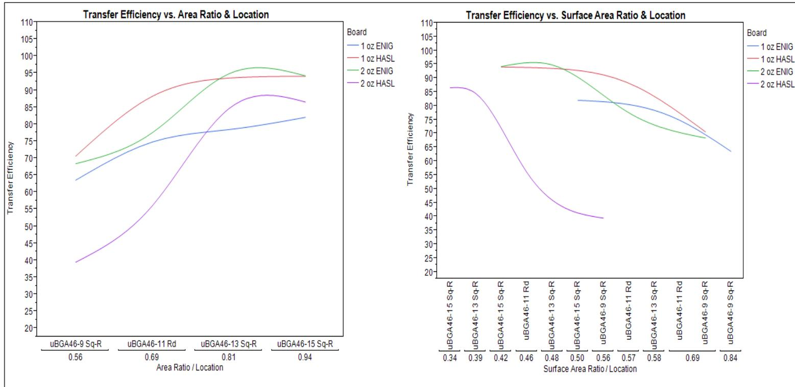
Calculating surface area ratio based on copper weight of the outer layer and the surface finish on the board is not a good method to predict transfer efficiency.
