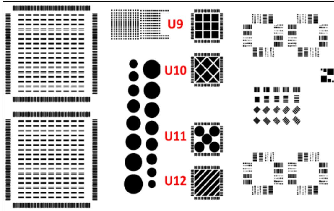
Stencil Design used to determine void percentage based on ground pad stencil design.
