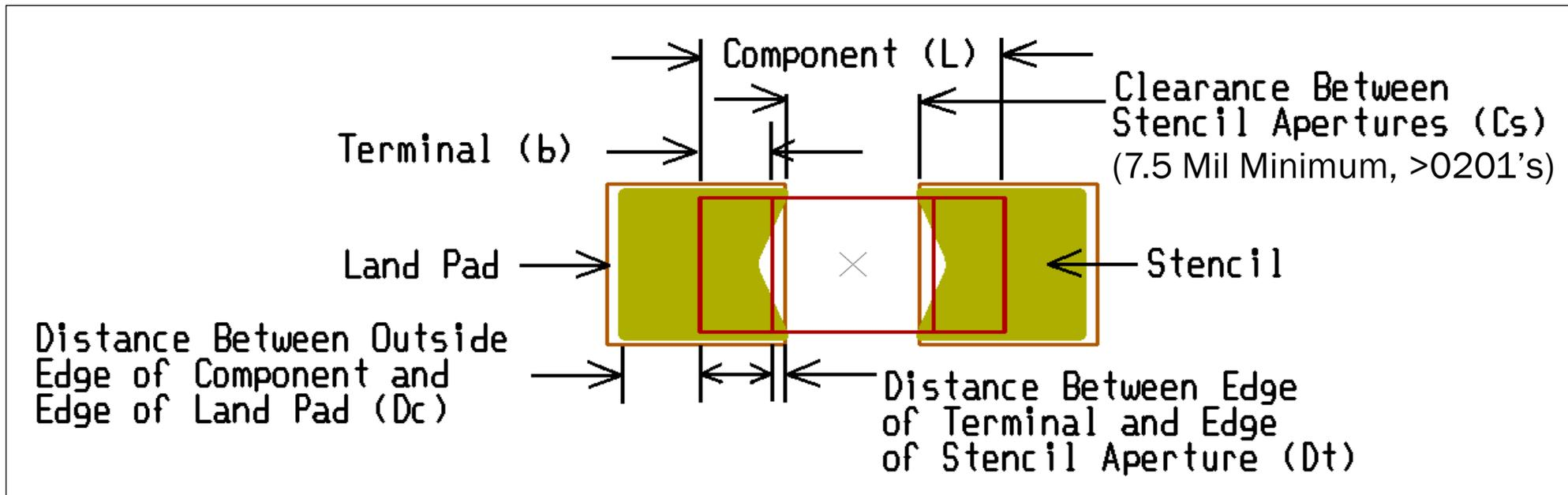
**ALWAYS CALCULATE AREA RATIO WHEN CHANGING TO U SHAPE OR INVERTED HOMEPLATE APERTURES**
