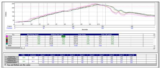
Figure 7 – Linear Ramp to Spike (RTS) Reflow Profile
