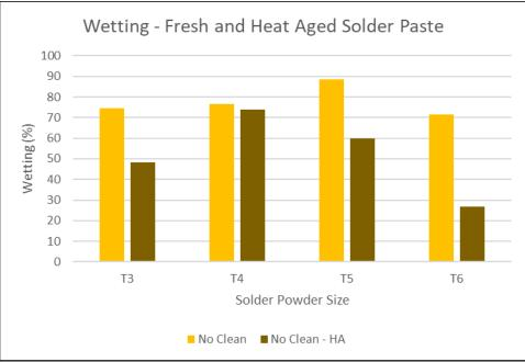
Figure 33 – Wetting for the No Clean Solder Pastes Before and After Heat Aging
