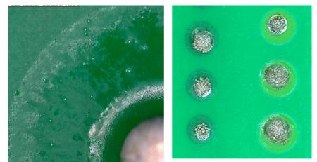
Figure 4 – Random Solder Balling (Left) and Graping (Right)
