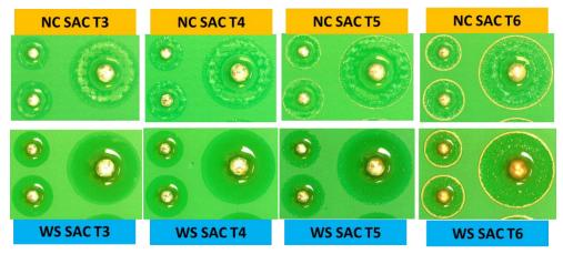
**Figure 23 – Solder Balling in the Overprint Patterns**
