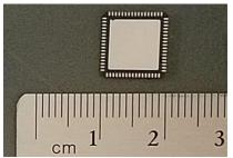
Figure 13 – QFN (MLF68) Dummy Component
