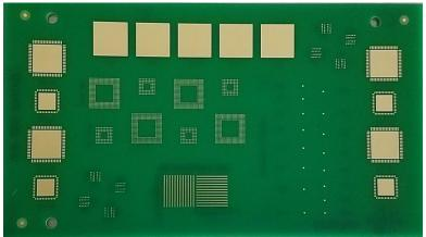
Figure 6 – Print and Reflow Test Circuit Board
