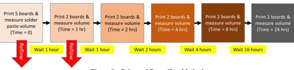
Figure 9 – Print and Pause Test Method
