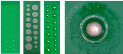
Figure 11 – PR Test Board Solder Balling / Pullback Patterns
