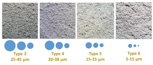
Figure 2 – IPC Type 3, 4, 5 and 6 Solder Powders
