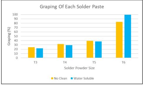
Figure 24 – Graping for Each Solder Paste
