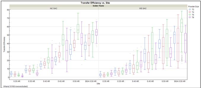
Figure 18 – Transfer Efficiency Box Plots for Each Solder Paste by Area Ratio
