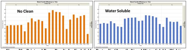
Figure 20 - Print and Pause Results for Each Solder Paste. No Clean (Left) and Water Soluble (Right)
