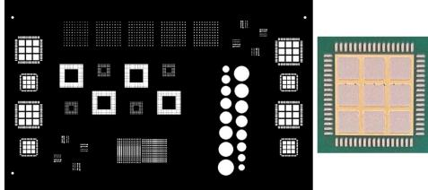
Figure 14 – Stencil Design for QFN Thermal Pads
