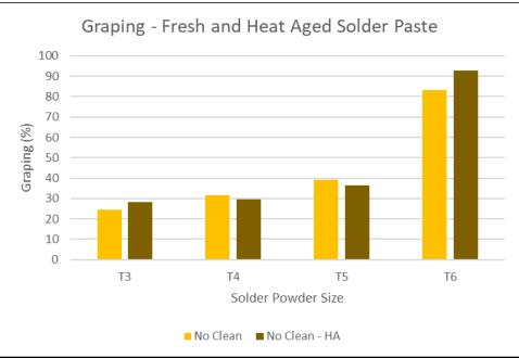
Figure 35– Graping of the No Clean Solder Pastes Before and After Heat Aging
