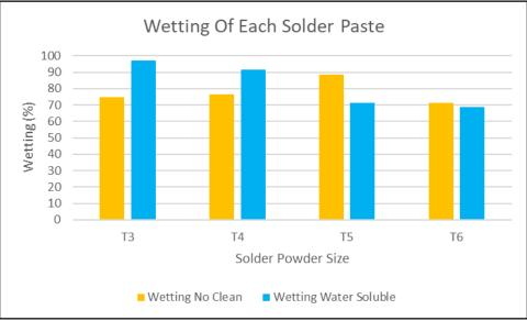
Figure 21 – Wetting or Spread of the Solder Pastes
