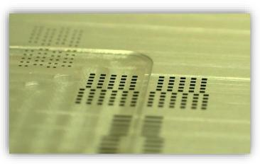
**1.1.7 Relief Etch** Also known as Etch Relief and Under Etch. Adding an under etch of the foil to create a pocket for raised features, labels, or a mulit-print function.
