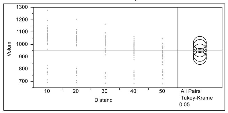
Tukey-Kramer HSD Analysis for the Uncoated, Welded 2.5 mil Step and the 9.8 x 35.4 Aperture.
