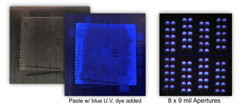
The printed solder paste volume is higher for the 10 and 20 mil distances than the 50 mil distance for the 9.8 x 35.4 mil apertures but smaller aperture volumes seem to be consistent from 10 - 50 mils from the step edge.
