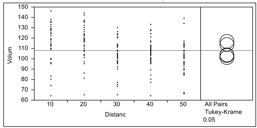
Tukey-Kramer HSD Analysis for the Uncoated, Machined 2.0 mil Step (2 mil step down) and the 8 x 9 Aperture.
