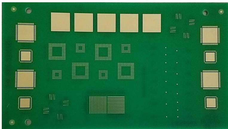
**Figure 6 – Print and Reflow Test Circuit Board**
