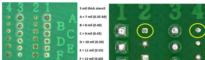
**Figure 12 – PR Test Board Graping Patterns**
