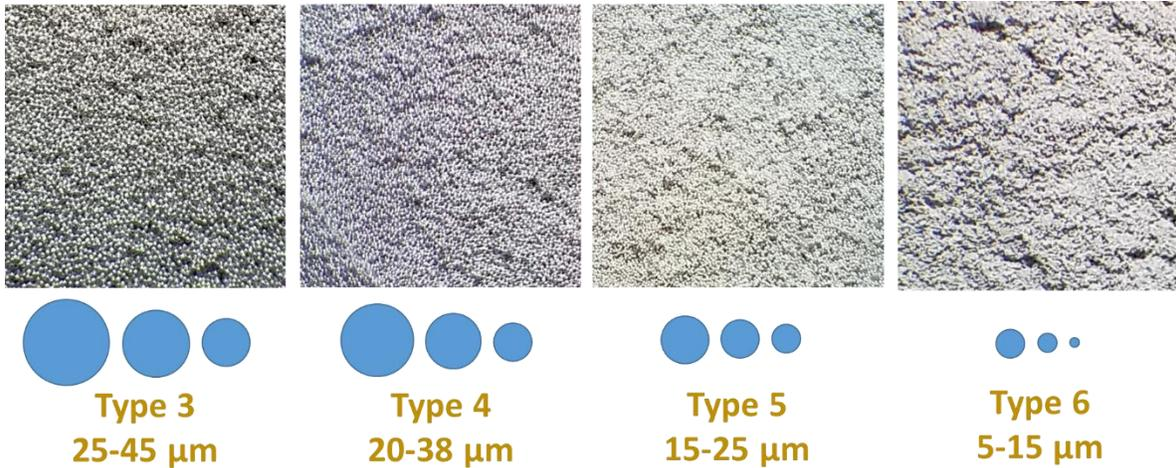
**Figure 2 – IPC Type 3, 4, 5 and 6 Solder Powders**
