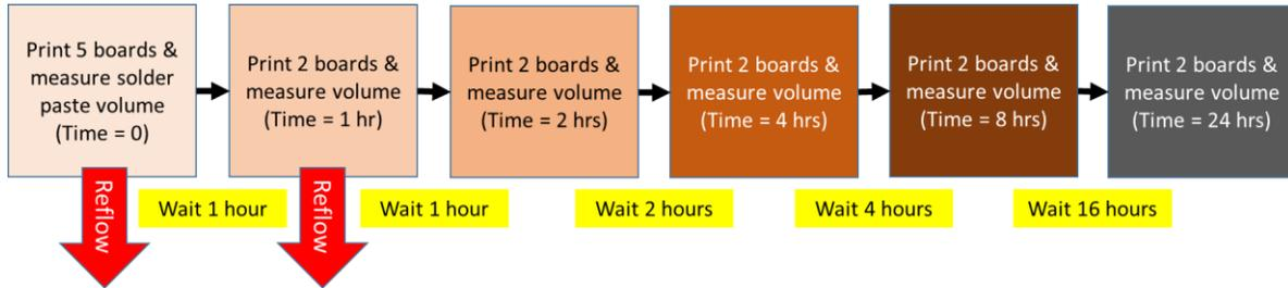
**Figure 9 – Print and Pause Test Method**
