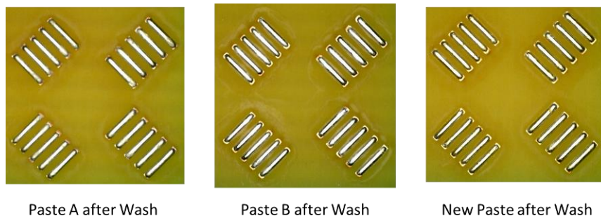
Figure 13 – Flux Residues on Circuit Boards after Washing
