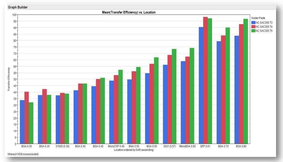
Solder paste: No Clean SAC305 Type 3, 4, 5. (Uncoated stencil)
